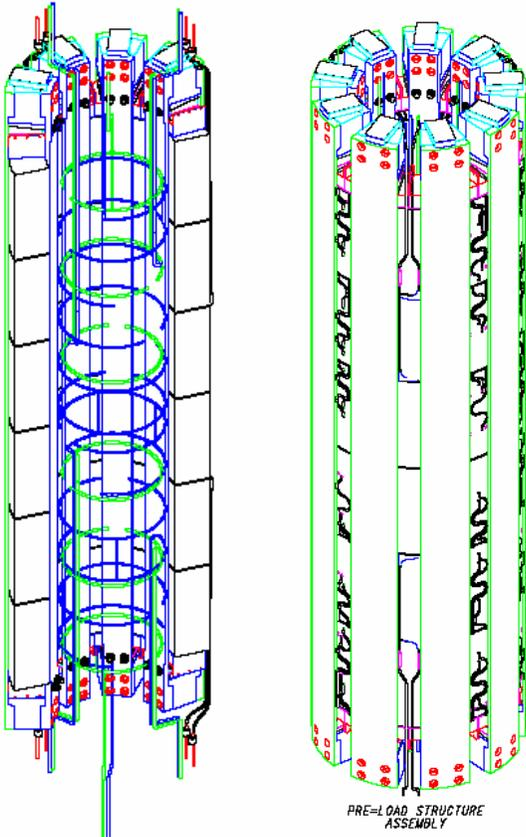
Fig. 5: Inner and outer coolant lines, current leads and preload structure assembly
