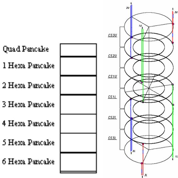
Fig. 4: Pancake module and lead arrangements in Central Solenoid
