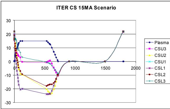
Fig. 2: CS Currents (MAT) vs. Time (s) for ITER 15 MA Scenario
