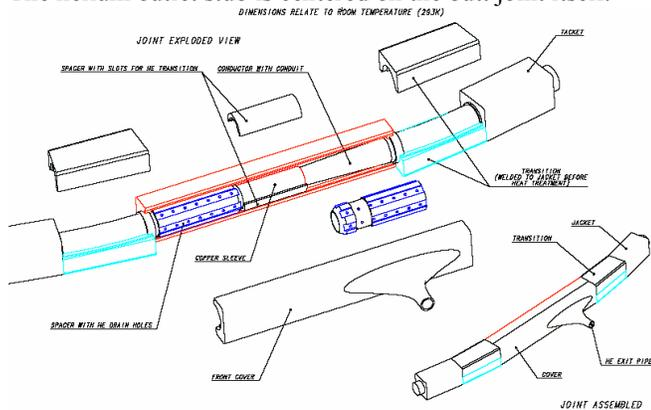
Fig. 7: Intramodule butt joint
