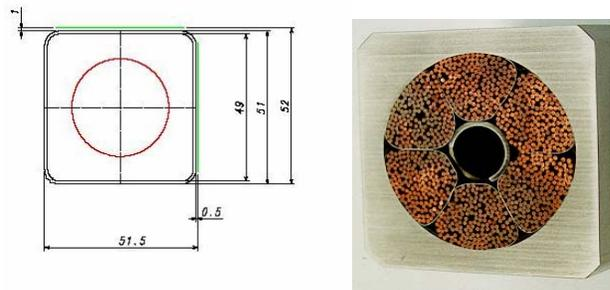
Fig. 6: CS Cable-in-conduit (CIC) superconductor
